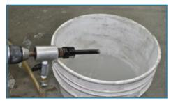
**Step 1** Attach the water swivel (central water feed) and wet core diamond bit to the drill. Connect the water swivel to a water source and adjust the water flow to a slow trickle. Constant, slow water flow will reducing chipping by cooling and lubricating the drill bit.
