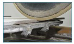
**Step 2** Adjust the blade height so the blade cuts through ù of the cement board thickness.
