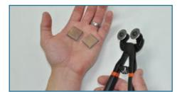
Glass mosaic tiles may also be removed from the sheet and wet cut individually or cut by hand using glass mosaic nippers.
